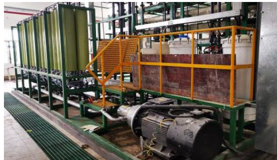
废水零排放 (DHP13.5, 60bar)
